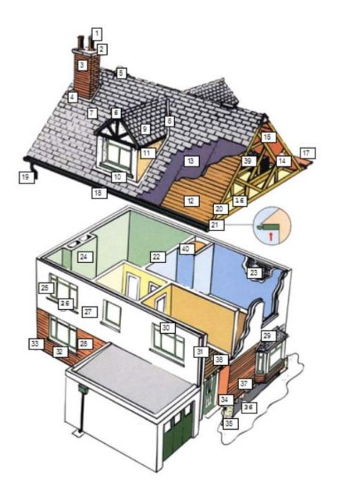
Flashing 4 Ridge ventilation 5 Ridge board Slates/tiles 8 Valley guttering 9 Dormer projection Dormer flashing 10 Dormer cheeks 11 12 Sarking Roof felt 13 Trusses 14 15 Collar 16 Insulation 17 Parapet gutter Eaves guttering 18 Rainwater downpipe 19 20 Verge boards / skews 21 Soffit boards 22 Partition wall Lath / plaster 23 24 Chimney breast 25 Window pointing Window sills 26 Rendering 27
